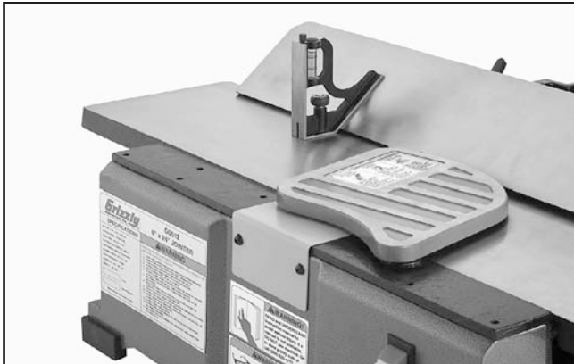
Figure 30. Checking the outward 45° stop.
